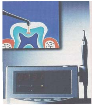
Figure 2- The red diode laser light is shone into a tooth surface free of
